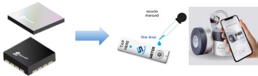
The chip can be used for smart labeling systems to prevent product counterfeiting, with customers being entrepreneurs aiming to add value and enhance product security. It can also be used to monitor various sensor readings, such as water contaminants, glucose levels, hormones, and viruses, aligning with the trend of digital healthcare.
